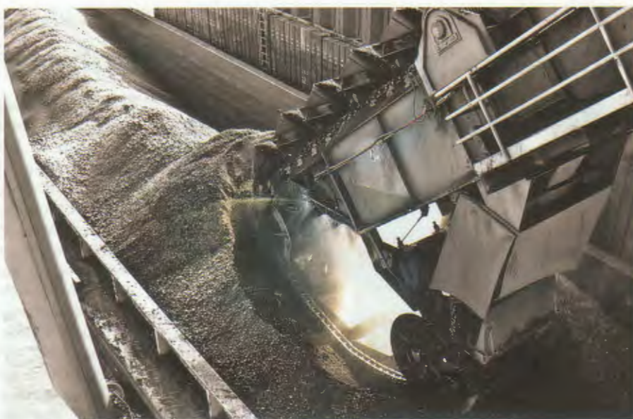
It is important to catch the dust at the point of emergence.
